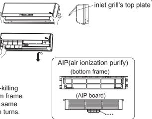
Note:the green aspect of the bacteria-killing medium air purifying filter will face outside, the white aspect will face to the machine. The yellow aspect of the VC layer will face outside, the white aspect will face to the machine.
